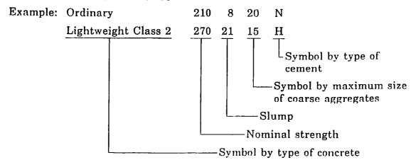
The symbols to be used for designating the ready-mixed concrete shall be as shown in Table 6 to Table 8.
